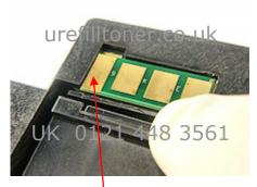
19) Press down firmly on top of existing chip with the longest contact plate on the left hand side as shown
